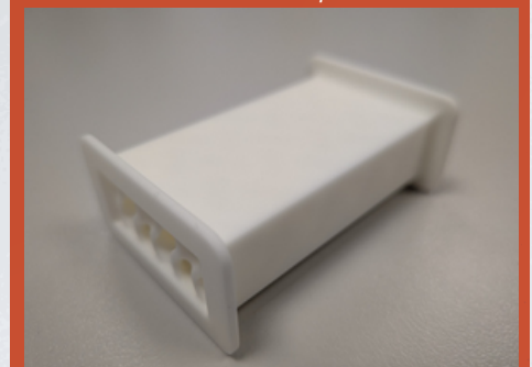
Coupon gyroid - 65% porosity, aluminum oxide, sintered
