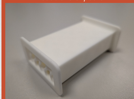
Coupon gyroid - 65% porosity, aluminum oxide, sintered
